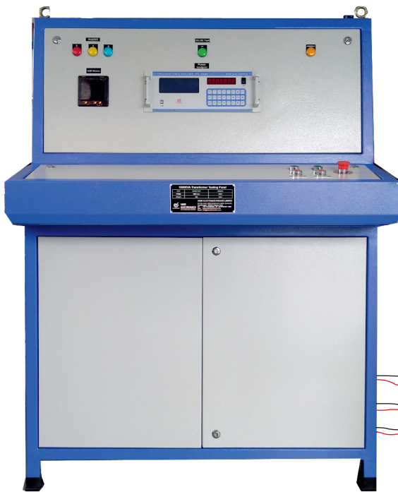
Pre Core Loss Testing Panel
